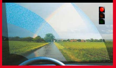
Deterioration of wiper blade linkage or decreased wiper pressure can leave parts of the windscreen unwashed.
