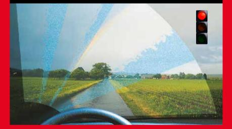
Deformed wiper rubber, worn linkage or wiper arm can cause juddering across the screen leaving behind radial streaks. Change your wiper blades and replace other parts as necessary.
