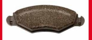
Appearance. Unequal wear pattern on the pad What caused it? No full contact between brake pad and disc, disc scoring by dust or excessive wear. New pads with a worn disc may also show this effect.
