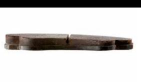
**Appearance.** Irregular wear or tapered pads What caused it? Distortion of the caliper and the slides are sticking and needless caliper clearance. What is the effect? Premature pad wear and noise while braking. Unequal braking pressure. How do you fix it? Replace pad set and maintain and service caliper. Note: some cars use pads that are tapered by design.
