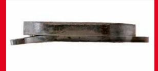
Appearance. A back plate that is damaged. What caused it? Not correctly assembled, or needless force used during fitting. What is the effect? Lower braking efficiency, irregular pad wear and braking noise. How do you fix it? Change brake pad set.
