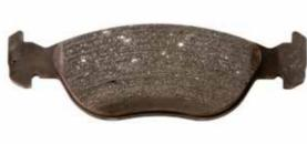
Appearance. Metal ingrained on the friction surface.
