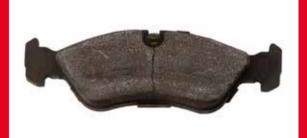
Appearance. Small cracks in the middle of the pad What caused it? Cracks illustrate that the caliper is sticking. The piston flexes the back plate causing the back plate to bend, cracking the friction material.
