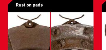
Appearance. Rust between the friction material and back plate.
