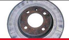
What caused it? Blue spots are a result of rising cracks caused by metallurgical change in the surface material making it hard and brittle. This is common in cases of overloading the brakes beyond normal design limits. This could result from aggressive driving, excessive payload or intensive/unusual brake use. What is the effect? Reducing brake performance, noise and vibrations.
