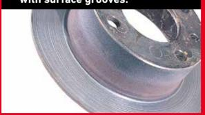
What caused it? Excessive or full brake pad wear results the brake pad backplate contacting the disc (metal to metal). This will make grooves in the disc surface.
