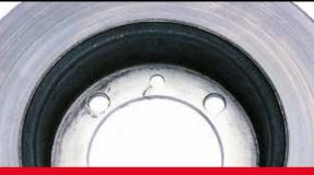
What caused it? Too much severe tightening torque used on positioning screw. What is the effect? Vibrations observed from the first brake applications onwards How do you fix it? Change discs avoiding excessive tightening torque. Positioning screws are just expected to ensure that the discs are positioned correctly.
