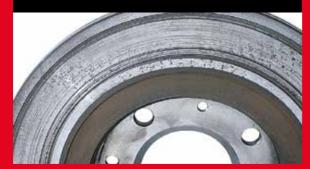
What caused it? Loose rough/sharp particles like dirt, road or water. Or badly mixed friction material between pads and disc.
