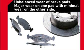
What caused it? One brake pad is in constant contact with disc
