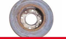
What caused it? Friction material deposits on disc surface. This usually appears where bad quality brake pads have been installed.
