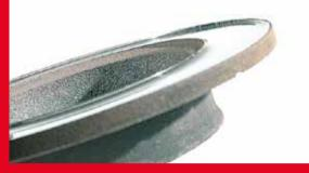
What caused it? Discs were not inspected regularly or replaced at the correct moment. What is the effect? Lower performance, excessive noise and vibration while braking
