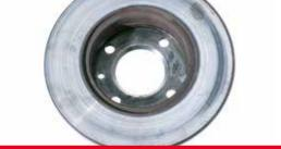
What caused it? Excessive hub run-out and uneven disc-to-pad contact generates vibration that causes localized heat.
