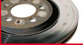
What caused it? Incorrect assembly of the caliper and/or pads can cause the pads being at a different angle to the disc, each side wearing at changed rates. Blue spots are generated by severe localized overheating. What is the effect? Progressive onset of vibrations, due to heat spots. Probable reducing of the brake efficiency. How do you fix it? Inspect and repair caliper. Replace pads.
