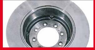
What caused it? Tightening sequence incorrect, not enough tightening torque used. What is the effect? Vibration on initial brake applications.
