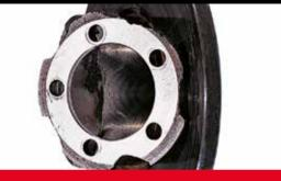
What caused it? Needless tightening and failure to observe recommended torgue and sequence by the manufacturer during tightening
